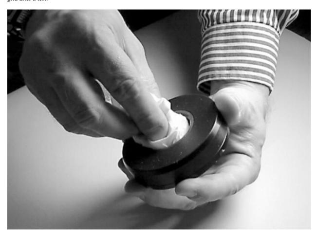
After the grid is wiped clean, apply a few drops of the next oil to be used onto the surface of the grid and wipe it clean and dry. This procedure is intended to "wet out" the surface of the sensor with the next oil, completely removing any trace of the previous oil. Make this double cleaning a standard practice as it prevents cross contamination of samples and is very important to reliable data collection.
